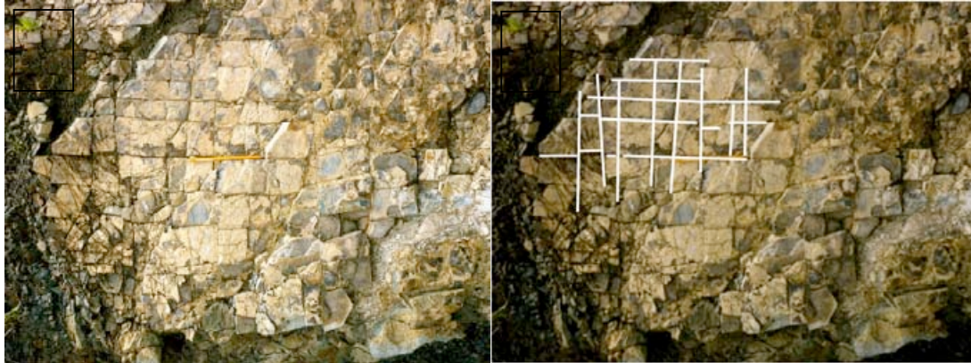
Figure 4.30 A & B: Jointing in the volcanoclastic bedrock in the headscarp. Note: yellow pencil for scale.
