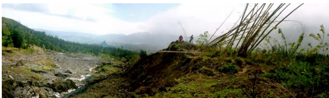
Figure 4.27: Image of the toe of the landslide facing northeast. Showing the last of the mid slope benches with a backwards tilt of 10^{\circ} south followed by a large scarp. Areas of large alluvial deposits with a newly formed stream can be seen in the left corner of the image. Upright vegetation also with backwards tilt essentially ‘surfing’ the slide. Note people at scarp edge for scale.
