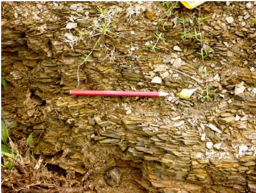
Figure 4.29: Bedded mudstone bedrock, the main component of the landslide colluvium.
